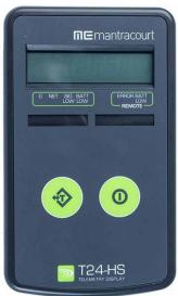
The T24-HS handheld display is a simple and easy to use 8-digit LED telemetry display providing one to one data display from a single T24 telemetry acquisition module (strain, current, voltage). Input values are transmitted to the handheld via 2.4Ghz radio allowing users to view a digital reading at distances of up to 800 metres.
