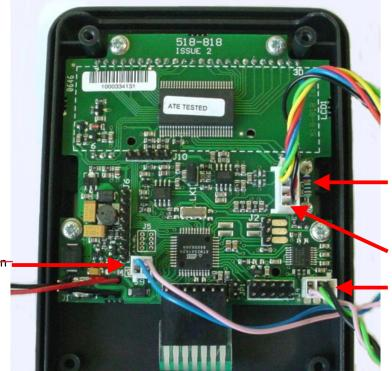
Shunt Calibration Resistor
