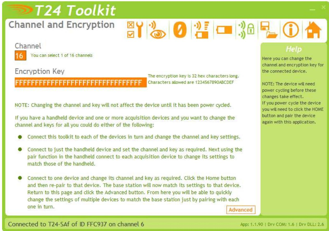
Here you can change the channel and encryption key for the acquisition module device. Simply pair to the T24-SAf and change its channel and key.
