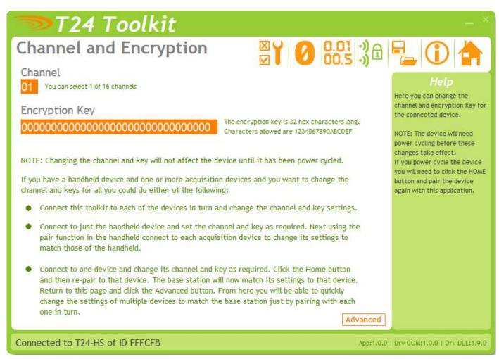
Here you can change the channel and encryption key for the acquisition module.
