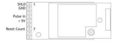
The 'Pulse in' input incorporates a pull-up resistor enabling a 'volt-free' contact to be used as the input source. This can take the form of a normally open or normally closed switch or relay contacts.
