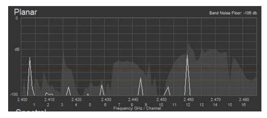
This shows a good RF environment. The Band Noise Floor is low and there are no red traces indicating that there are plenty of signal free gaps to enable T24 to transmit. There is traffic across the whole band with higher signal traffic between channels 11 to 15, but there is nothing that would affect T24 operation.
