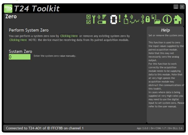
System zero allows you to zero the input. The system zero value is subtracted from the input value before it is used to determine the analogue output to apply.
