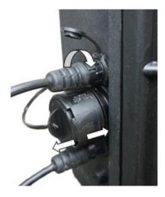
The PP1 110 Vac – 240 Vac input has a sealing cap for when it is not connected to the mains. The sealing cap is removed by pushing the outer sleeve towards the case and pulling the cap out.
