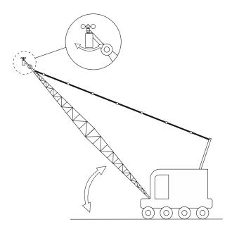
d. The entire wind speed sensor should be located so that the cups are fully exposed to the wind and so that the sensor rotates freely at all boom angles. Avoid mounting the sensor where objects have created wind turbulence.
