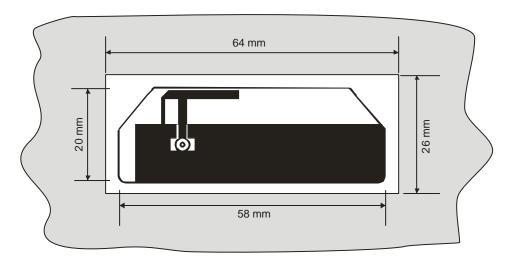
The antenna feeder cable, or any other cables or wires, must not be routed over or near the cross hatched area shown below as this will affect range.
