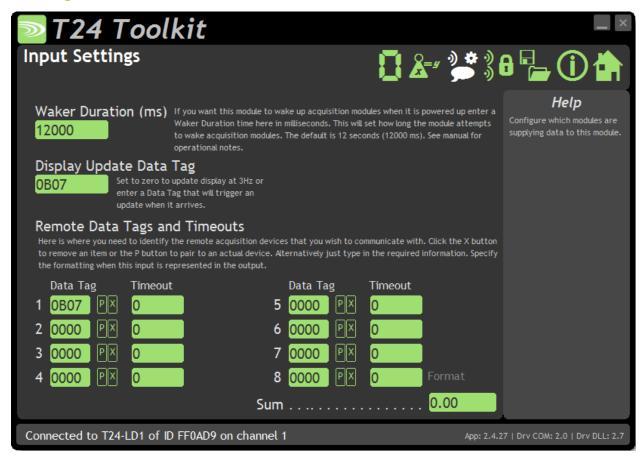
Use this page to enter the Data Tags of the T24 transmitter modules to be summed and displayed on the T24-LD1. The user can also set the Data Tag that will trigger a display output along with how the data is formatted.
