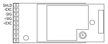
The resistance of the strain gauge can be between 85 and 5000 ohms. The T24-SA can support up to four 350 ohm strain gauges bridges attached in parallel (At the expense of reduced battery life).
