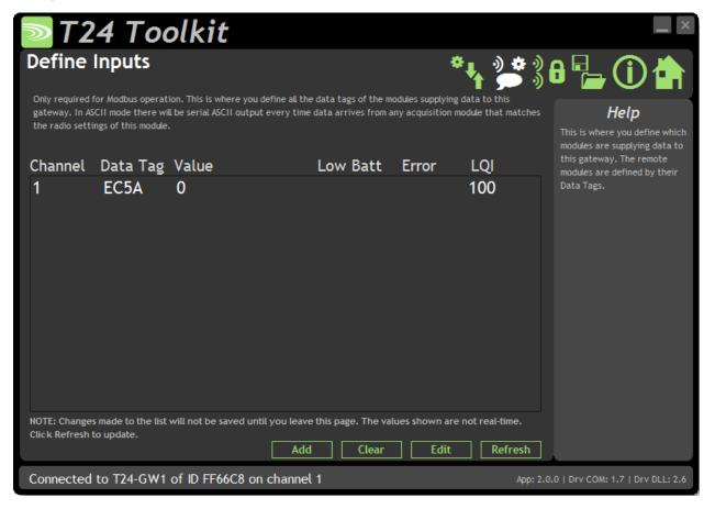
This is where you define which transmitter modules are to be providing data to this module when in Modbus mode.
