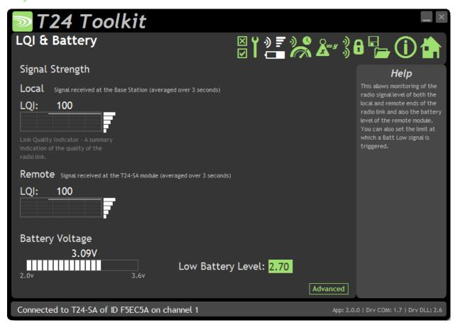
Here you can see the voltage of the battery and the radio signal levels at the base station and the remote transmitter module. This simple view gives an LQI value which stands for Link Quality Indicator. This value will range from 0 to 100 and within this band you should still achieve communications. As the level drops towards zero communications may become intermittent but still achievable.
