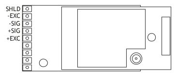
The resistance of the strain gauge can be between 85 and 5000 ohms. The T24-SAf can support up to 4 350 ohm strain gauges bridges attached in parallel (At the expense of reduced battery life).
