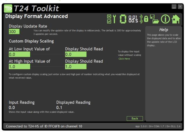
Here you can adjust the display update rate and also scale the displayed data. This may be used, for example, to convert the data from a T24-SA calibrated in kg so that the handheld display shows lb.
