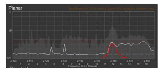
This shows how the display would look if the band noise floor slowly crept up. The red trace is only visible on channel 12 but other channels that were once OK (Having a very low minimum signal level) now have a viewable level of minimum signal noise. A double-click on the planar chart would reset the peak and minimum calculations so the minimum red trace would then follow the more recent higher noise floor.
