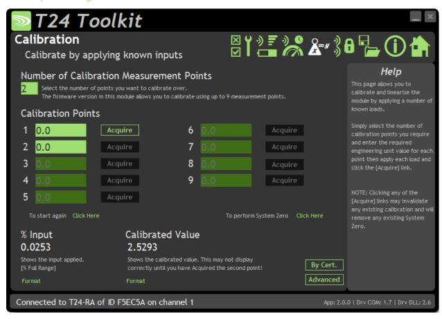
The module is factory calibrated to provide between 0% and 100% output value when the positive input varies between the negative and positive excitation.
