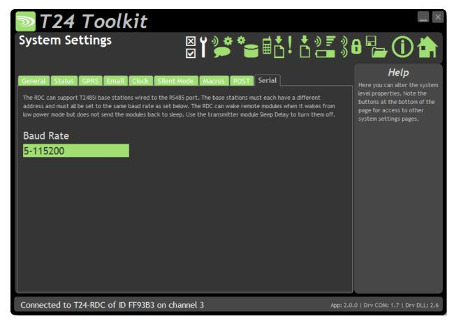
The RDC can support locally wired serial T24-BSi base stations connected to J9 configured as RS485.
