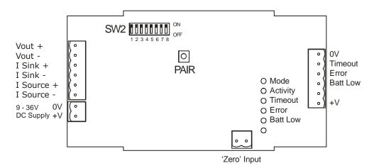
The LED indicator states are also represented on open collector outputs as seen on the right hand connector in the above diagram. They draw no current when the state is inactive and are conducting when the state is active.
