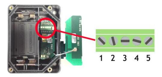
The input connections are accessed by lifting the right hand cover plate, this plate incorporates the T24-ACMi Antenna; take extra care when re-assembling that the grey UHF cable is attached to the antenna socket.
