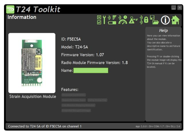
Once successfully paired to a module this page is displayed showing you information about the connected module.
