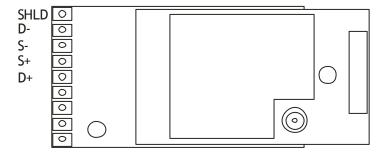
The Pt100 probe can be connected in 2, 3 or 4 wire measurement configurations.
