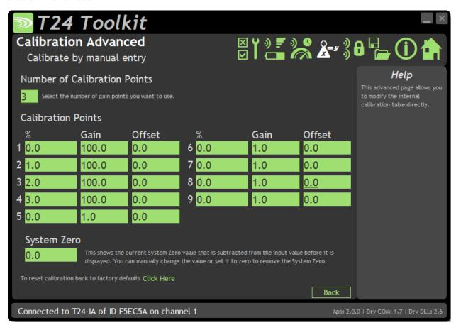
In some circumstances it may not be possible to apply inputs in which case the calibration can be entered manually.
