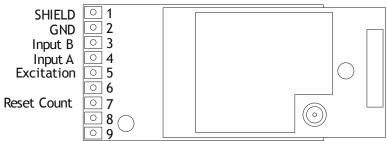
The 'Input A' input is used for Frequency, RPM, Interval, Counter, Digital State and Mark output types. This can take the form of a normally open or normally closed switch or relay contacts. The input resistor selection of pull up or pull down can be selected to suit the input.
