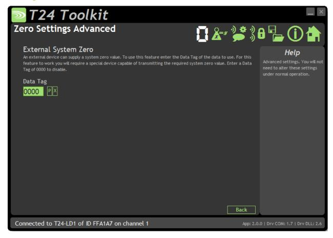
This advanced section allows the use of a specially configured external module to supply the system zero value.
