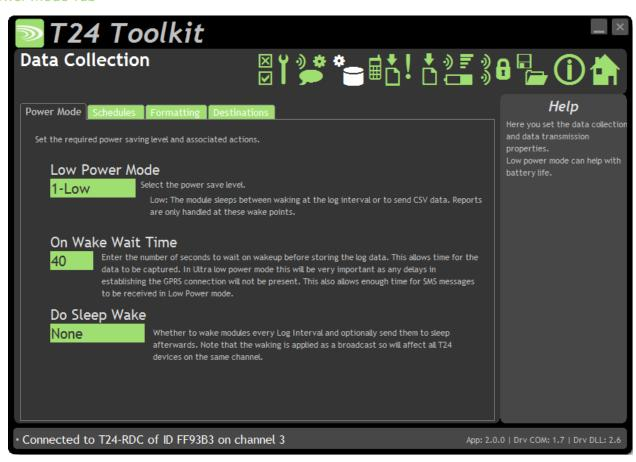
Here you define the how the data is collected and when and also determine how the CSV file is formatted and where it is delivered to. The Power Mode tab lets us change the following.
