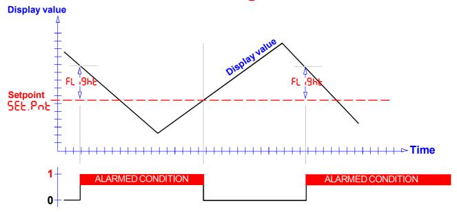
The Setpoint can be placed anywhere you like, in the range 89999 to +999999 and will include a decimal point in the appropriate position if you have set your display range to have a decimal point.
