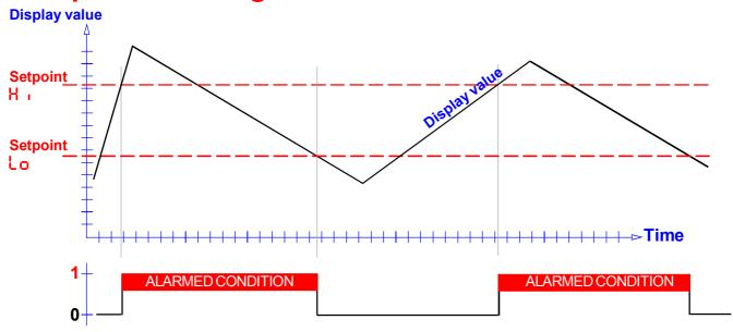
The Setpoints can be placed anywhere you like, in the range \$9999 to +999999 and will include a decimal point in the appropriate position if you have set your display range to have a decimal point.
