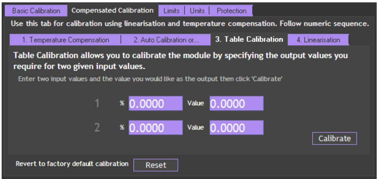
This option lets you calibrate direct from the sensor manufacturers certificate without having to apply inputs to the module.
