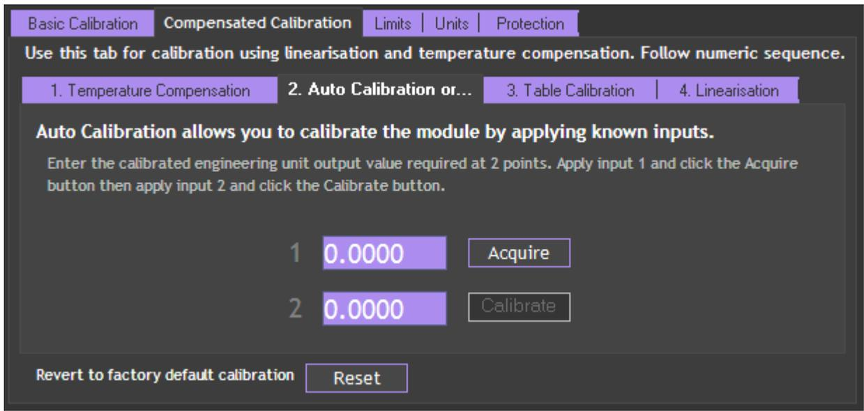
The automatic calibration requires that you apply two known (ascending) inputs in sequence. Just enter the required engineering unit value for the two inputs in the fields marked 1 and 2.
