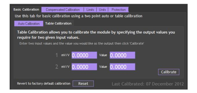
This option lets you calibrate direct from the loadcell manufacturers certificate without having to apply weights to the input.
