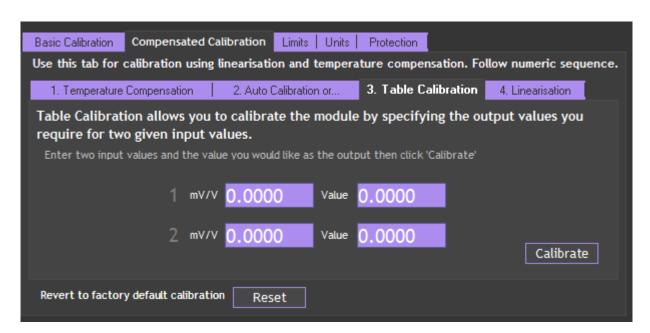
This option lets you calibrate direct from the loadcell manufacturers certificate without having to apply weights to the input.
