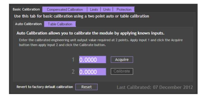
The automatic calibration requires that you apply two known (ascending) weight in sequence. Just enter the required engineering unit value for the two weights in the fields marked 1 and 2.
