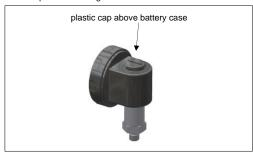
To change the batteries, go ahead as follows - this has only to be done in switched-off condition
